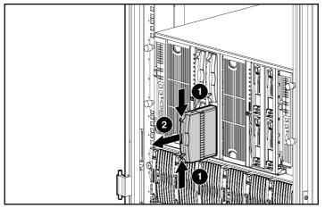
Figure 1-21: Removing a hard drive blank
